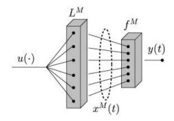
**Figure 1:** A: Architecture of a LSM. A function of time (time series)  $u(\cdot)$  is injected as input into the liquid filter  $L^M$ , creating at time t the *liquid state*  $x^M(t)$ , which is transformed by a memory-less readout map  $f^M$  to generate an output y(t).
